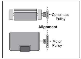
Figure 71. Pulleys aligned.
